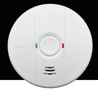
The PSA Lifesaver 6800 model is a mains powered, 9V battery backed smoke alarm. The alarm uses photoelectric technology and is designed to be surface mounted on the ceiling or wall. It can be used as a single stand alone unit, or can be interconnected with up to 24 units.
