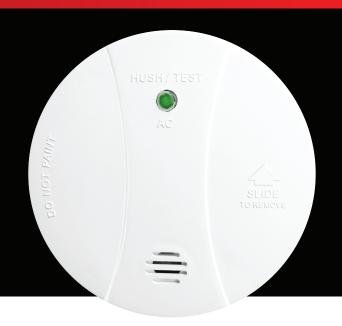
The HOMEGUARD HG3000 is a mains powered, photoelectric smoke alarm that operates on a 240VAC power source with a 9VDC battery backup. This smoke alarm has the ability to function as a stand alone unit or in an interconnected system. This smoke alarm uses photoelectric sensing technology and do not contain any radioactive material.
